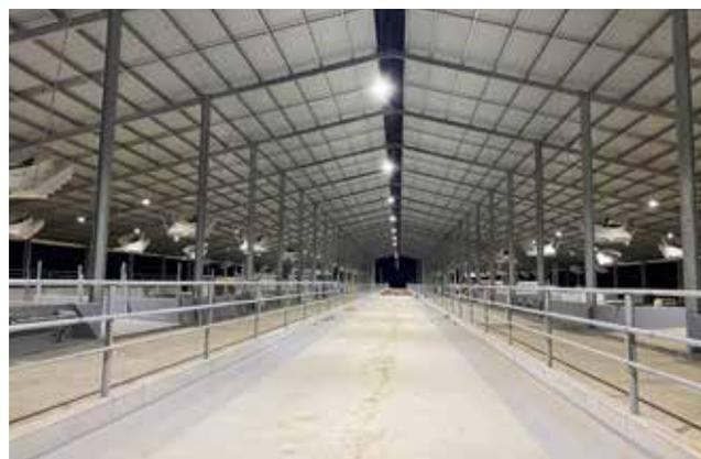
Cross overs between the feed and stall alleys should be located at the ends of each pen to avoid dead ends which inhibit cow flow.
