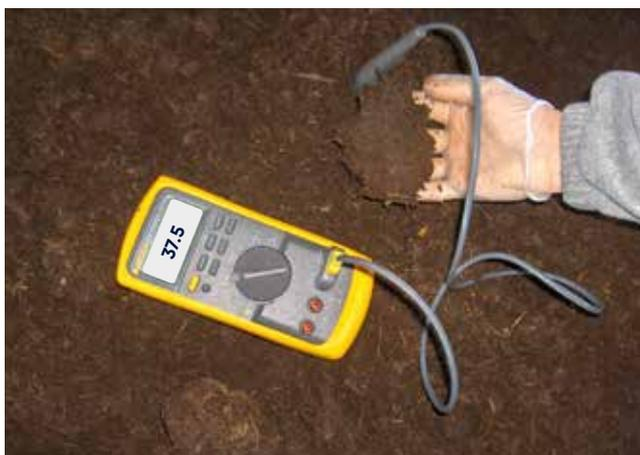
*C: Example of compost that is too dry with insufficient temperature – will not form ball*
