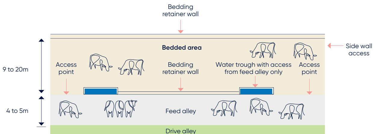
**Figure 35.** Concrete retaining walls provide separation between the feed alley and the bedded pack area which is helpful in managing pack moisture
