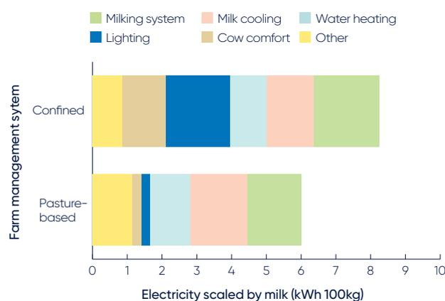
Note: Confined = Contained. Electricity use in kWh per 100kg milk broken down into the component of the dairy operation the energy is used in.
