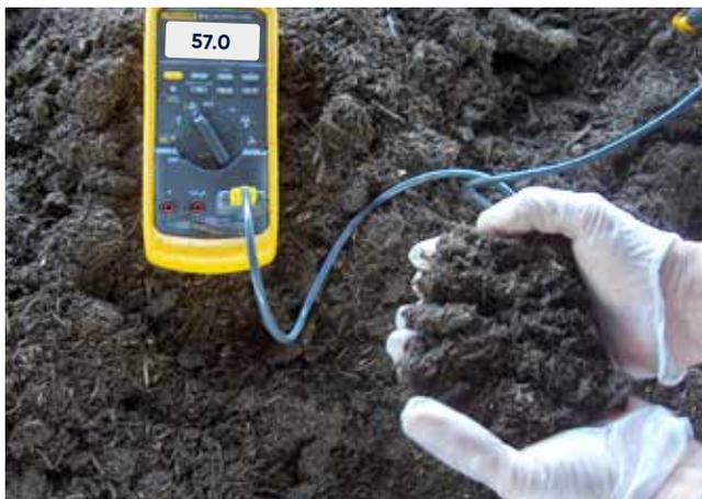
*B: Example of compost that is too wet with insufficient temperature – forms firm ball with water drops*
