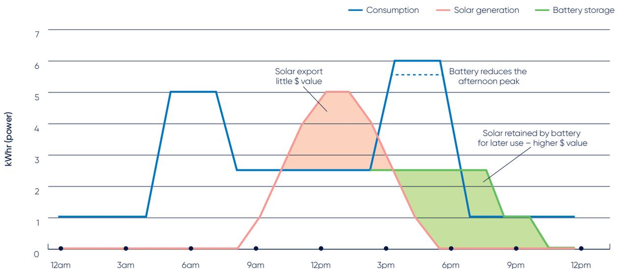
Note: Graph demonstrating how batteries can be utilised to capture energy for utilisation when there is increased demand.
