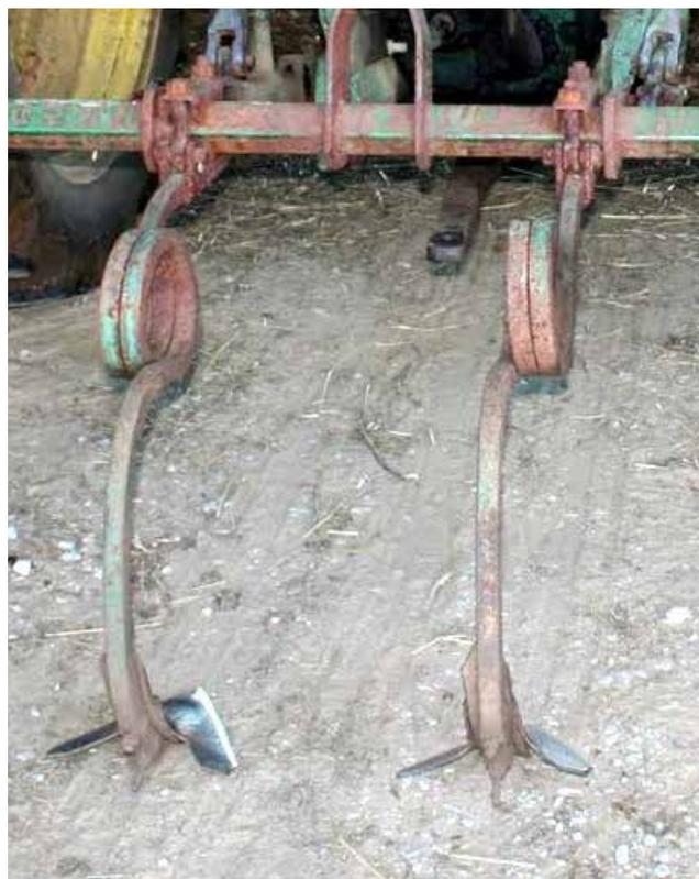
**Figure 48.** Roto-tillers may be used and are helpful to break up clumps of bedding material and maximize oxygen/air infiltration into the pack providing a uniform mix of material
