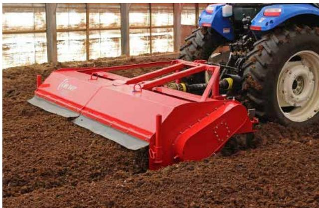
It is important to breakup tractor tracks by positioning mixing tools to follow the tires. If heavy equipment is used, wheel tracks will not be broken up; also, if the pack is too wet, the pack may become compacted, limiting oxygen and causing lower temperatures (Figure 49). Compaction prevents air infiltration into the pack, which is needed by composting bacteria. Compaction also leads to higher bed moisture and thus inadequate aeration.
