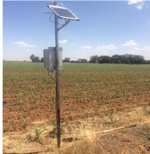
Cellular telemetry site with soil moisture probe connected.
