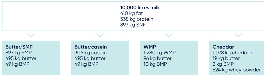
The milkfat and solids contained in manufacturing milk can be used to produce a wide variety of dairy products. There are four major production processes. The first two are for butter/skim milk powder production and butter/casein production which are joint product processes. The other two are whole milk powder production and cheese production. Furthermore, for each of these separate product lines, numerous other dairy products can be made from the residual milk components.
