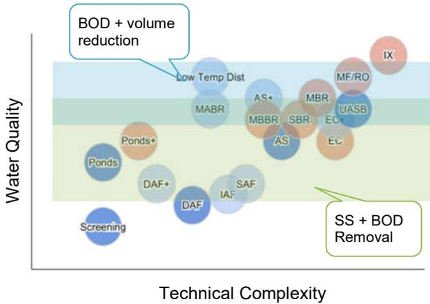
**Figure 8 Typical treatment technologies mapped by complexity against treatment ability**
