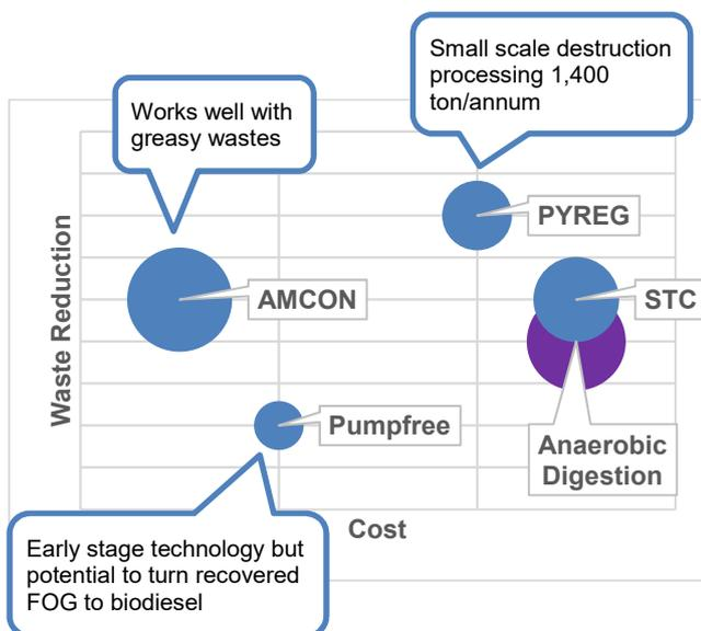
Figure 13 Mapping of sludge reduction technologies
