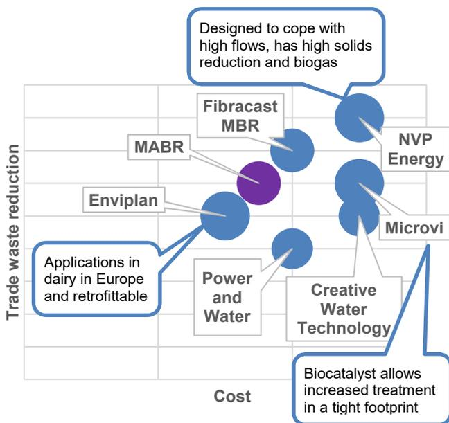
**Figure 10 Mapping of wastewater treatment technologies**
