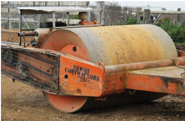
Vibrating roller for compacting laneway during construction of base layer
