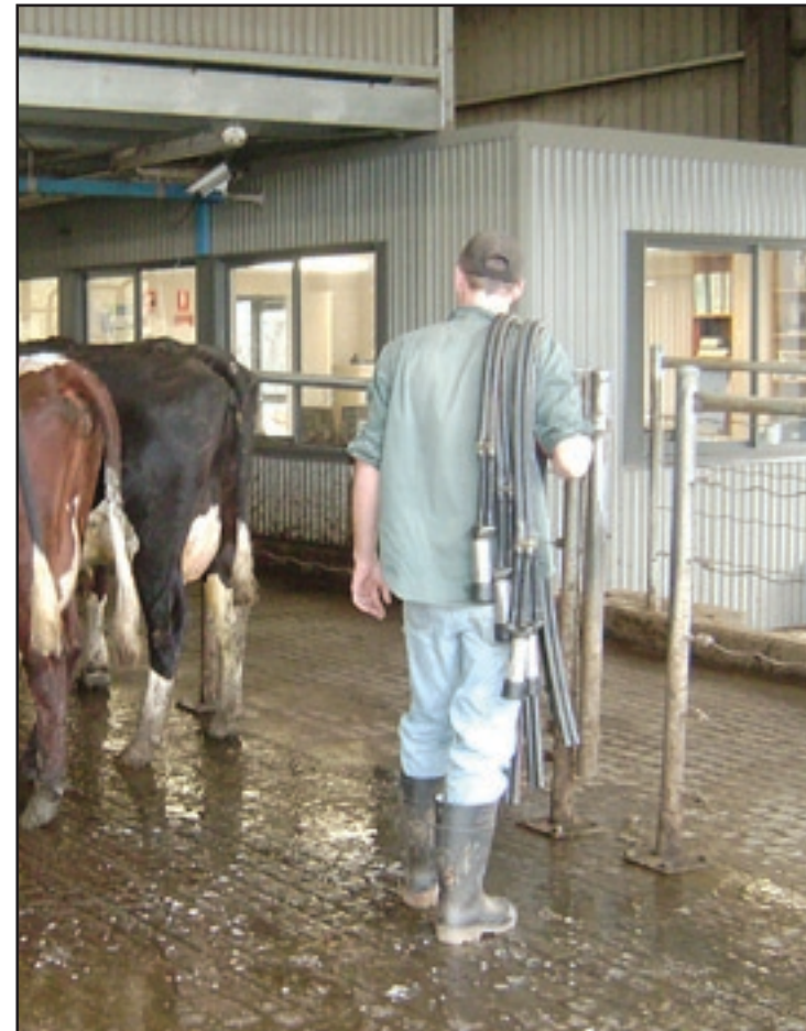
Changing liners and/or rubberware is a relatively quick task with an AMS, but should be done more frequently.
