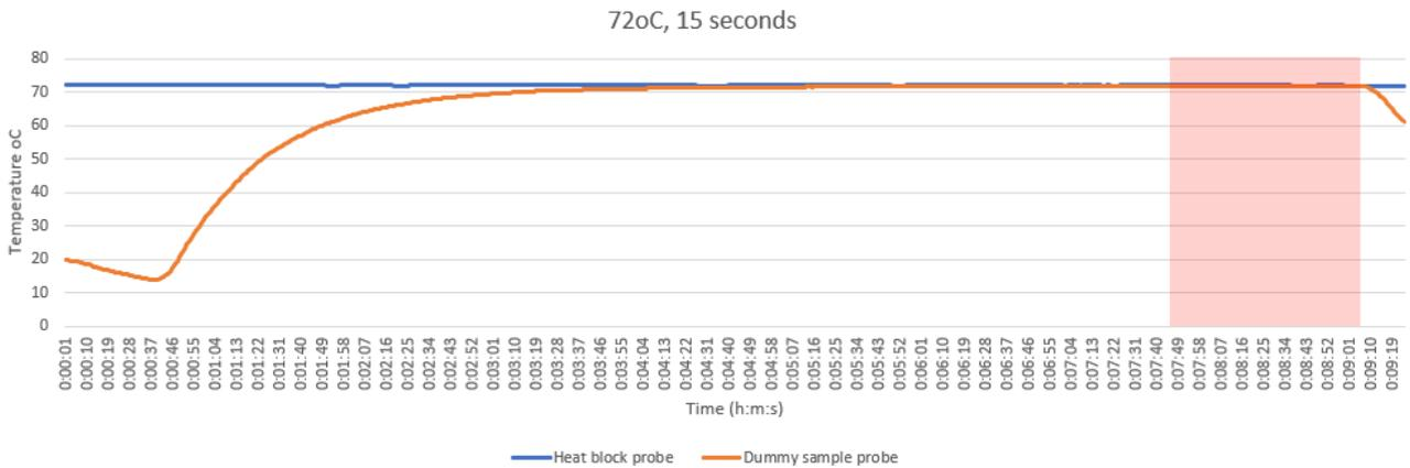
Figure 6. Temperature read out from the data logger files for the pasteurisation experiment. The blue line represents the temperature of the heat block, and the orange line represents the temperature of the dummy milk sample. The red box represents the period of time where the dummy sample reached the appropriate temperature, and spiking experiments were conducted in this time period.
