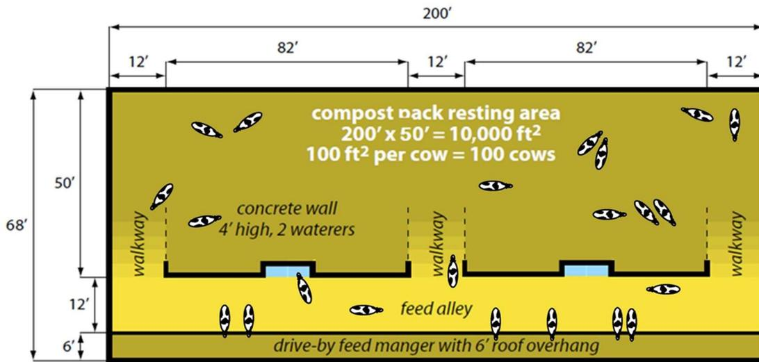
Figure 12; Minnesota type composting barn layout in USA, with concrete alleyway, watering troughs and fed bunk separate from the compost bed. Source; Endres et al. (15)
