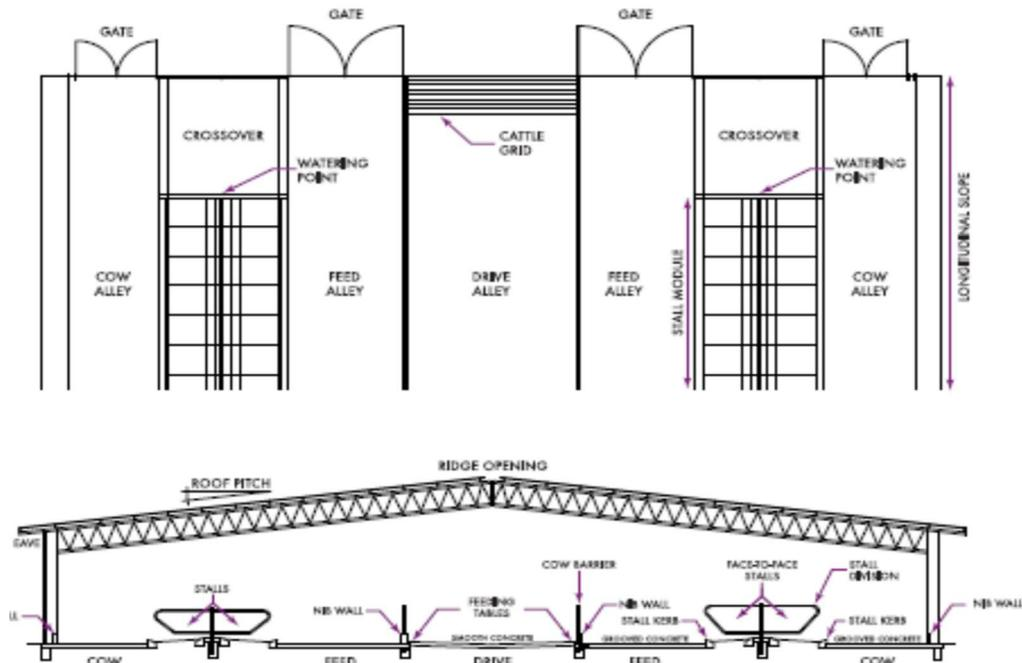
Figure 2. Freestall Design. *Guidelines for Victorian Feed-pads and Free-stalls*. Ed 1. 2010. Vic DPI (21)
