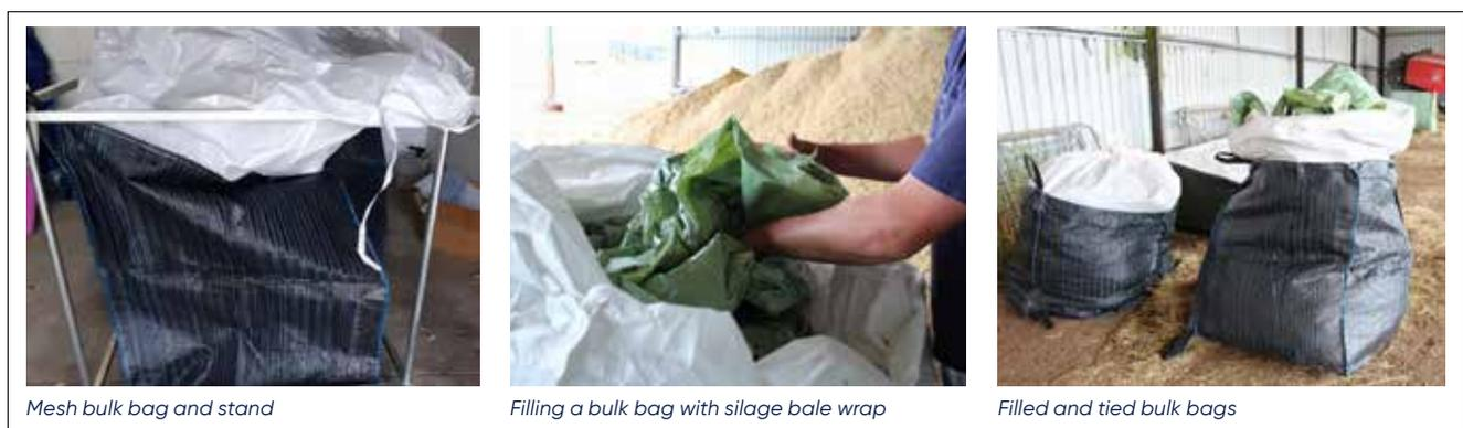
Figure 8. Ventilated bulk bag system.
